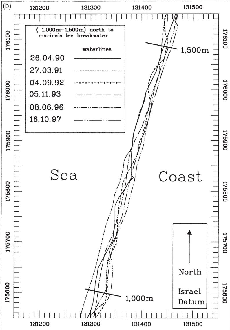
Fig. 3. (b) The waterline as shown on aerial photographs (1990–97) for the coastal segment 1000–1500 m north of the marina's lee breakwater.
